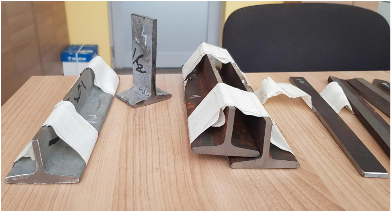
Figure 2 Structural steel sections for the mechanical testing (from left to right) ST-P2, ST-P4 (not tested), ST-P1 and ST-P3
