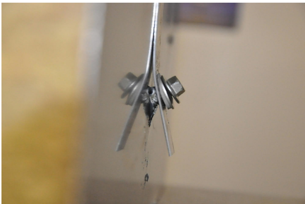
Figure 51 SL3 screw pull-out failure mode in shear tests.
