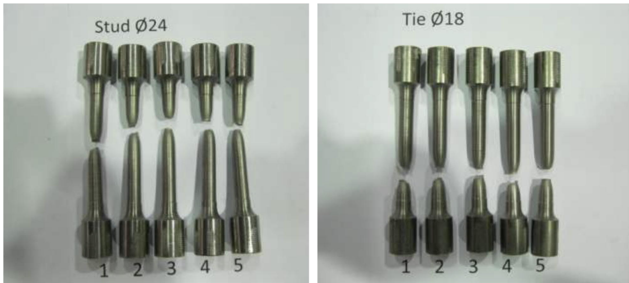
Figure 1 Tensile test specimens ST-B1 (first on the left) and ST-B2 (second on the right)
