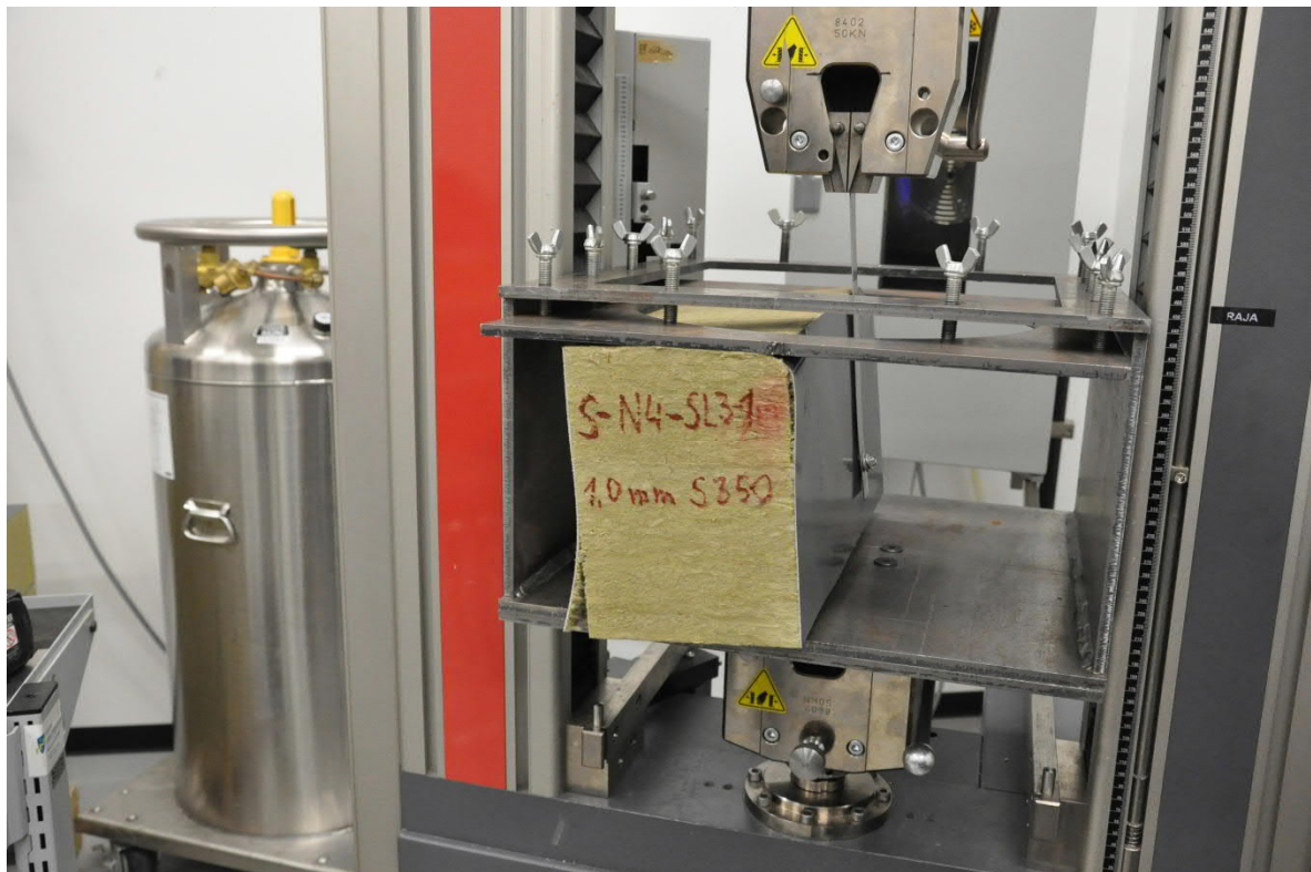
Figure 48 S-N4-SL3-1mmS350-1 panel condition during the test.
