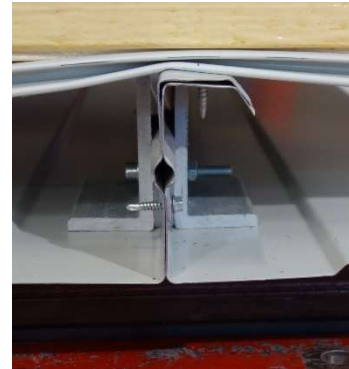
(b) Liner tray web after test
