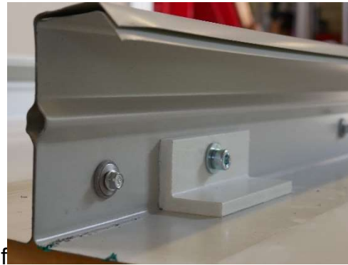
(b) Reinforcement of liner tray web
