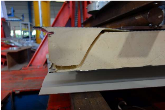
(a) Shear failure in core of sandwich panel
