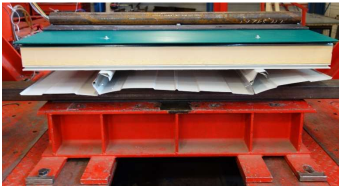
(a) Failure mode at the webs
