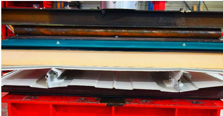
(a) Failure Mode at the webs
