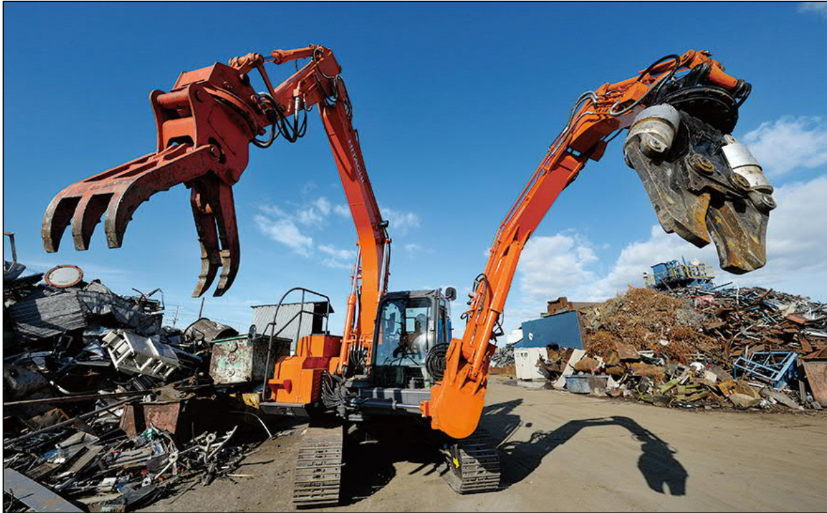
Figure 1.14 Hitachi two-boom excavator with grapple and steel shear attachments
