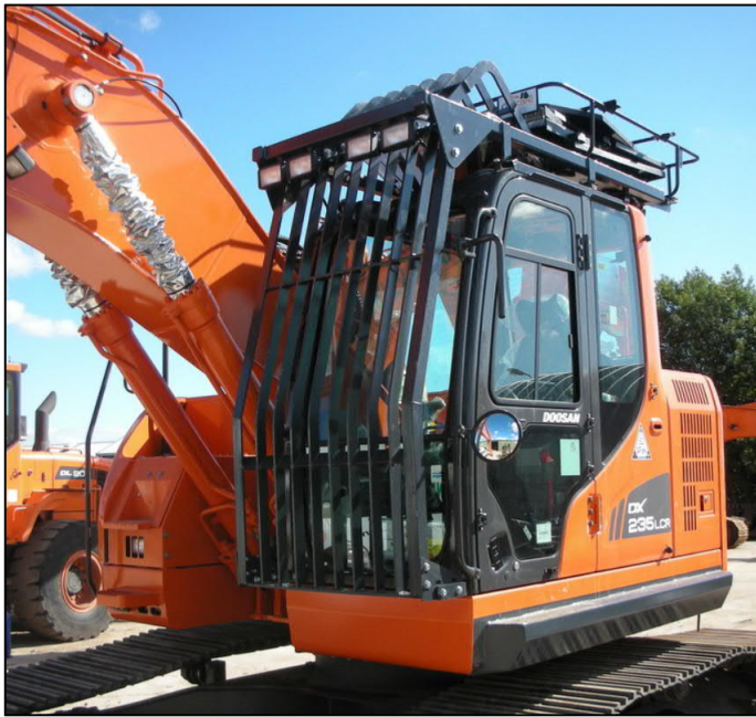
Figure 1.11 Falling object protection cage fitted to an excavator
