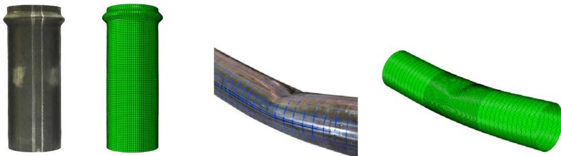
Figure 13: Typical experimental and numerical failure modes for stub column tests (left) and four-point bending tests (right)
