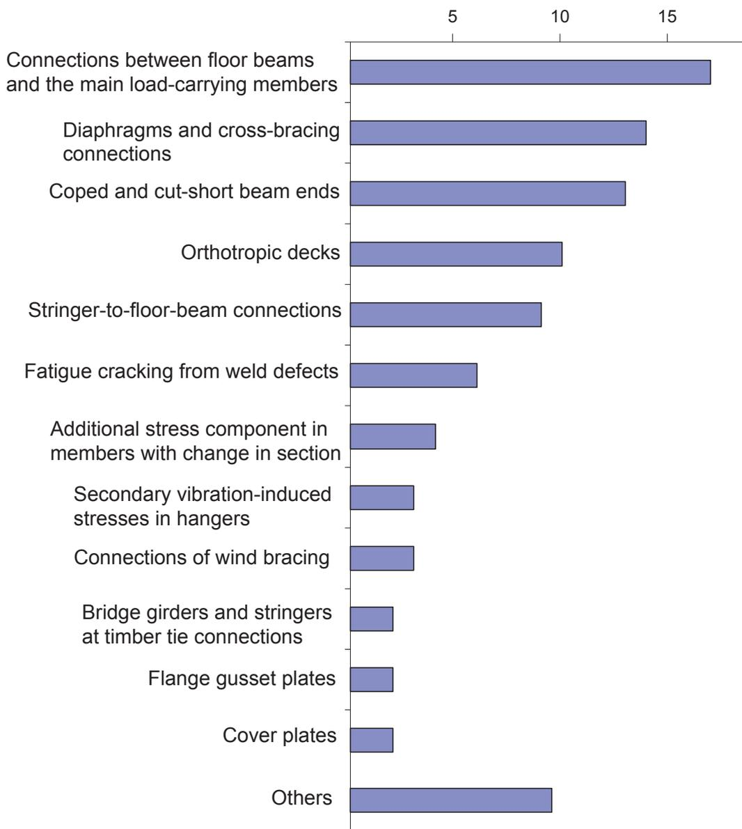
Fig. 1: Collected fatigue damage cases listed according to the type of detail in which they were encountered
