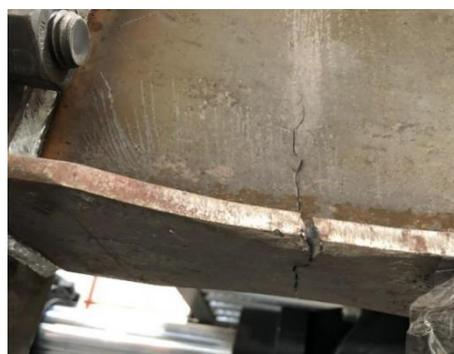
d) Failure at the centerline of RBS 1C
