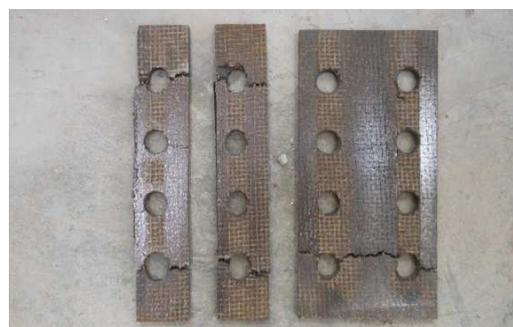
a) Test on Rubber M2 [43] 4 bolts – Preload level of each bolt 50 kN - 2 contact surfaces)    b) Brittle failure of rubber friction shims along the net section [43]
