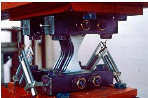
a) ADAS device after testing
