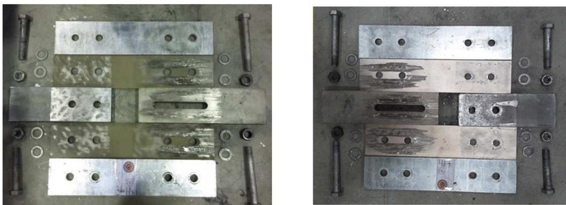
a) Damage of M6 shims
