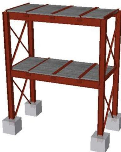
Figure 6.22 – 3D model of the mock-up with RBS connections
