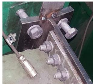
Figure 5.13 - Connection after failure: T-stub
