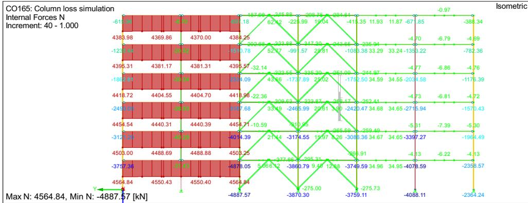
Figure 118. Normal internal forces in IPE600 frame after column loss (scenario 1)
