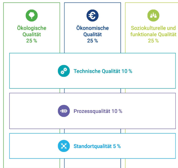
Figure 9: Basic structure of the DGNB System New Buildings
