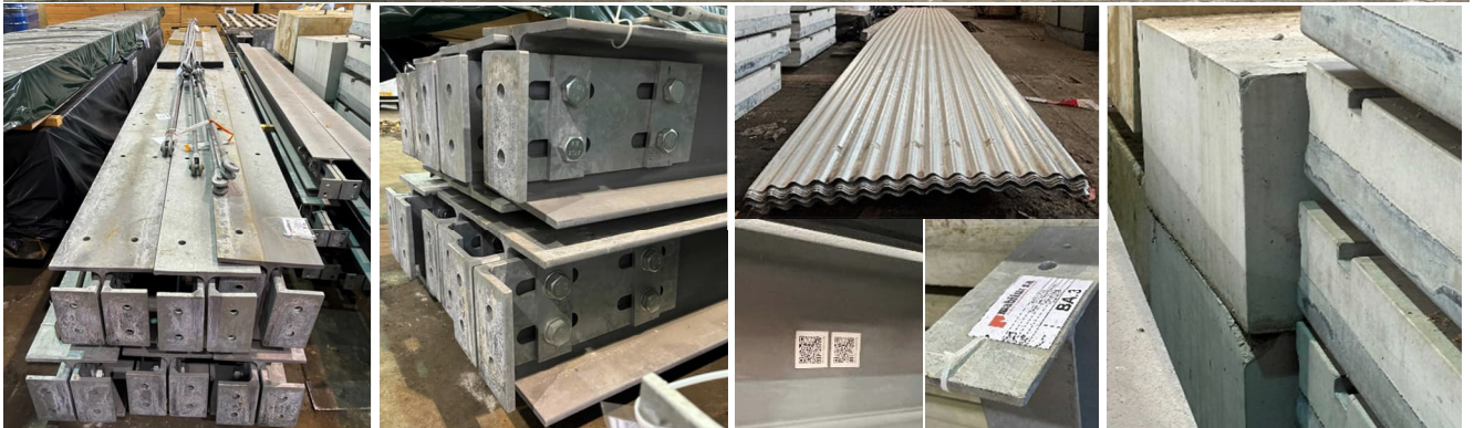
Reclaimed materials are stored at ArcelorMittal's Differdange site, with steel connections reassembled, and QR codes and labels attached to the main structure components. Local damages to the concrete foundation blocks have been observed.
